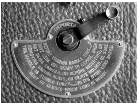
Crank with label on procedures for moving mirror and exposing the plates.
