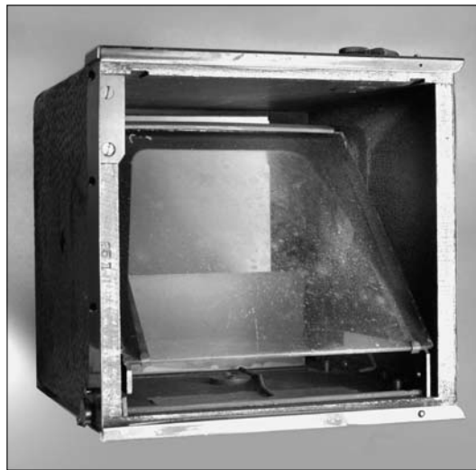
The large cam is revolved by the exterior crank and is seen at its halfway point where the wire with a hook, having caught the first plate, locks it in place on the floor of the camera. Then the yellow filter is brought down to 45° angle as part mirror and filter for the image.
