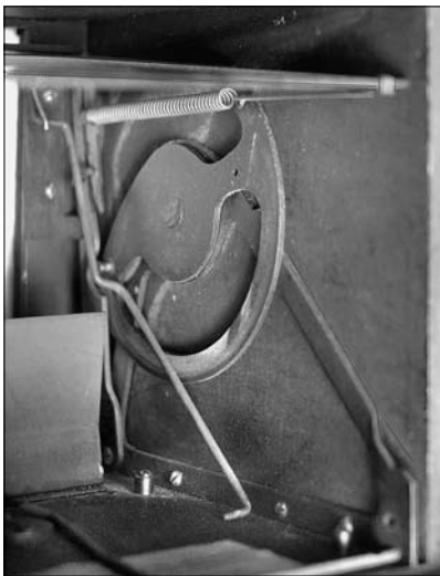
The large cam is revolved by the exterior crank and is seen at its halfway point where the wire with a hook, having caught the first plate, locks it in place on the floor of the camera. Then the yellow filter is brought down to 45° angle as part mirror and filter for the image.
