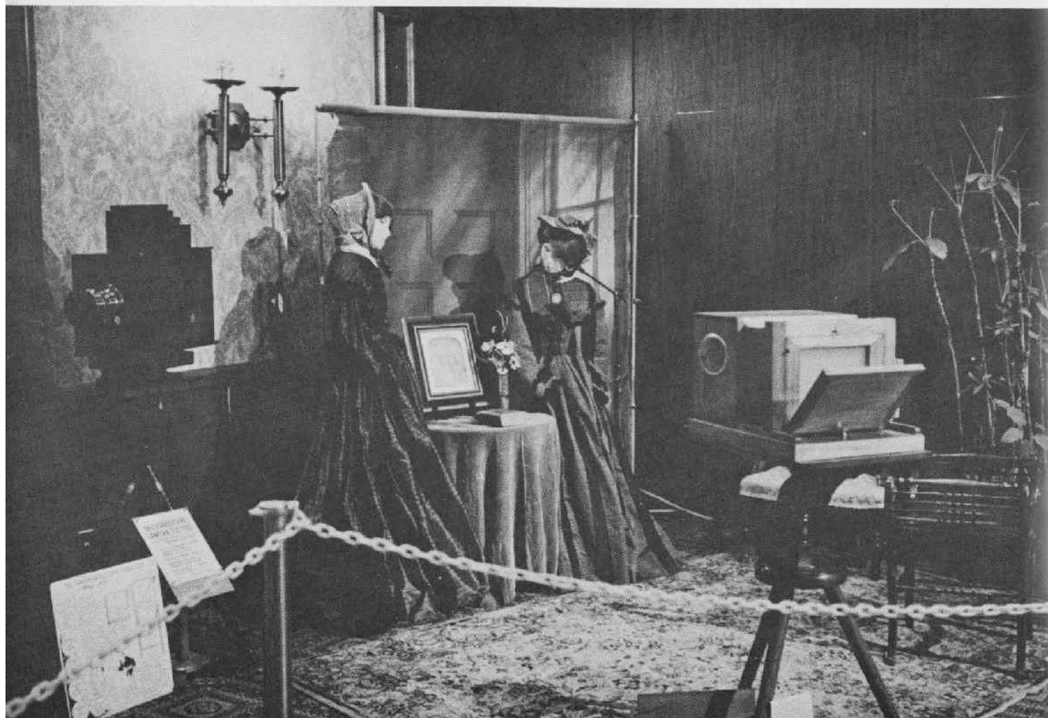
Fig. 1 Camera at left is an 8"x10" Roberts daguerreotype camera; at right is an exact replica of the 1839 whole plate Giroux daguerreotype camera.
