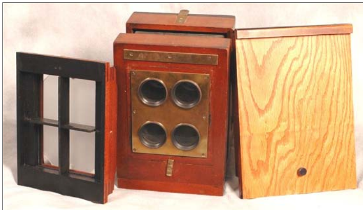
Left to right, modified back, camera, and flap shutter.
