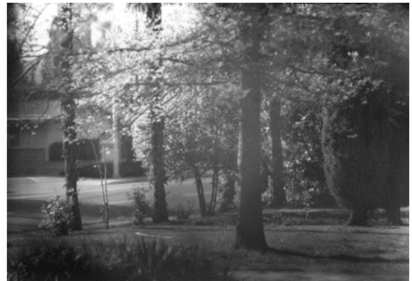
Zeiss Triplet flare when pointed near the direction of the sun.
