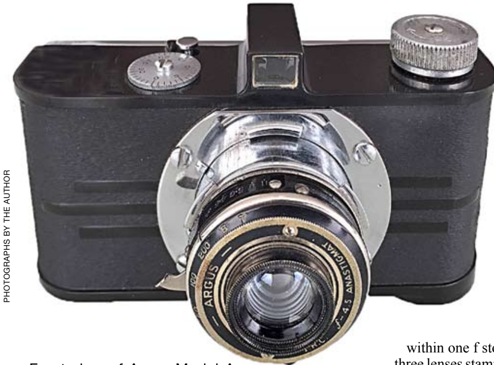
Front view of Argus Model A with Art Deco bakelite body.
