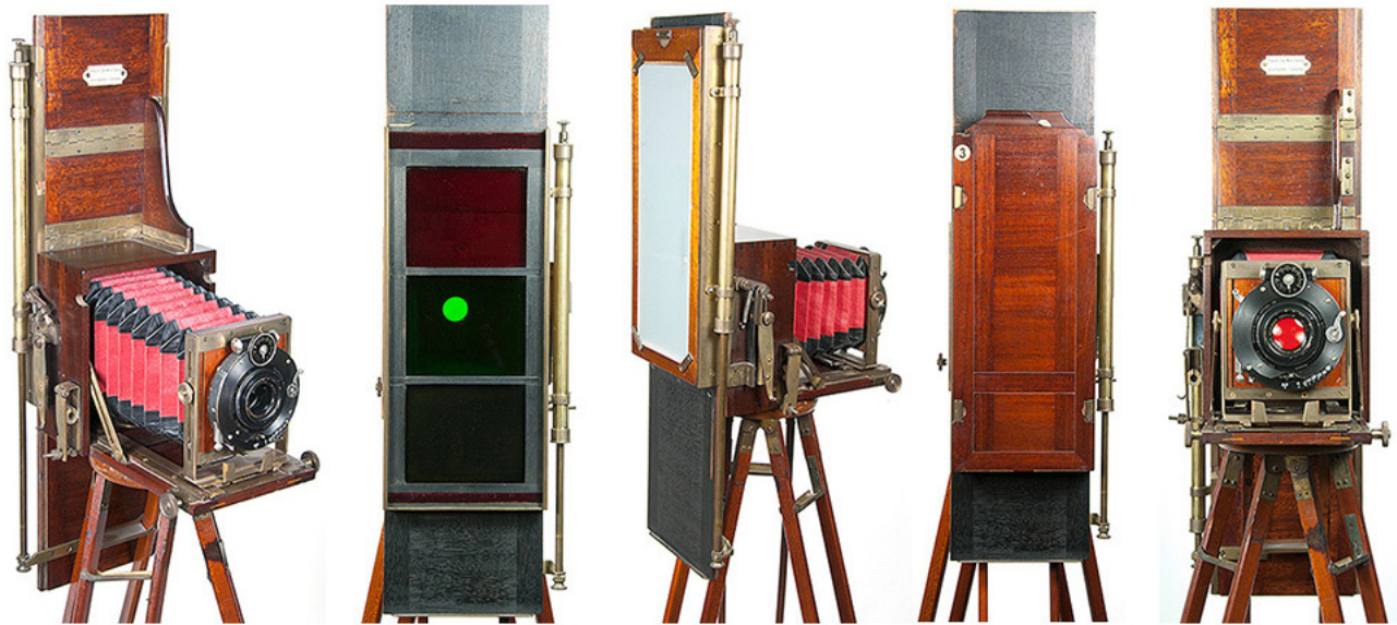
This three-color repeating back camera, ca. 1903, was designed by Dr. Adolf Miethe and built by Wilhelm Bempohl. Sergei Mikhailovich Prokudin-Gorskii's camera was either this model or similar and based upon this design.
