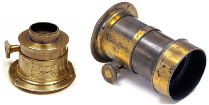
Figure 1. Typical landscape (L) and portrait (R) lenses. While the brass-work evolved over time, the optics remained essentially the same for decades.
