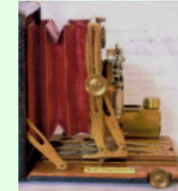
T. Curved arm at the front and a cranked arm behind
