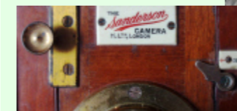
G. Lens-panel slots into a groove with a locking nut and is held by a small tag on the right-hand side.
