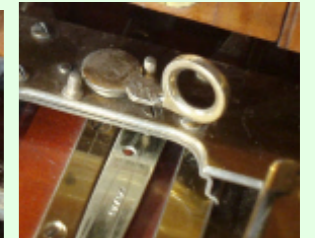
C. Locking with a thumb screw
