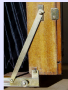
A. Hinged struts that locate into brass posts
