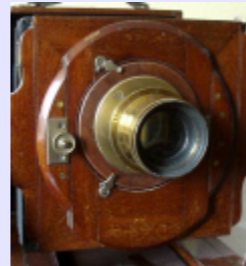
B. Circular with rack and pinion vertical movement
